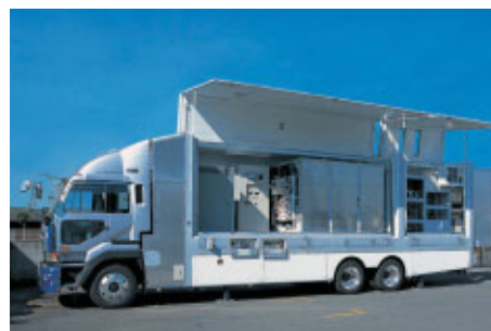
The hydrogen production and compression facilities are mounted on a truck
