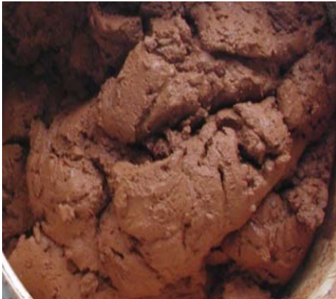
Excess sludge dehydrated with centrifugal dehydrator
