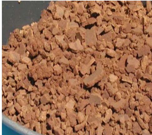
Sludge at left after dehydrating with electro-osmosis dehydrator
